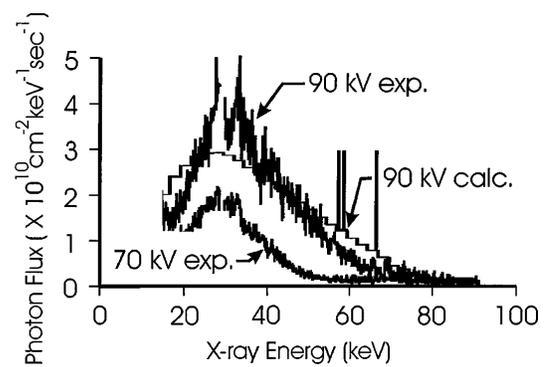
FIG. 1. Graph of the x-ray spectral flux expected in the position of the isomeric target. Rectangular steps plot calculated intensities normalized to the measured exposure. The experimental data for 70 and 90 keV end points were measured with a planar Ge detector from input attenuated with a pin hole and were normalized to the calculations.
