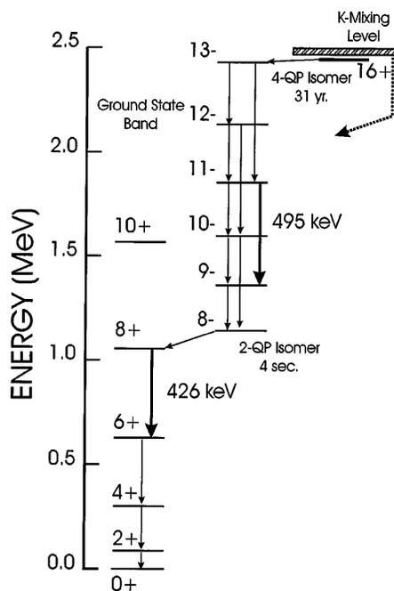
FIG. 3. Energy level diagram for  $^{178}\text{Hf}$  showing a selection of levels relevant to this experiment. The spontaneous decay of the 31-yr,  $16^+$  isomer is shown by the thin arrows. The thick solid arrows show components studied in this work from the particular cascade from the decay forced by the x-ray irradiation. Heavy dotted arrows are inferred transitions needed to feed those shown.
